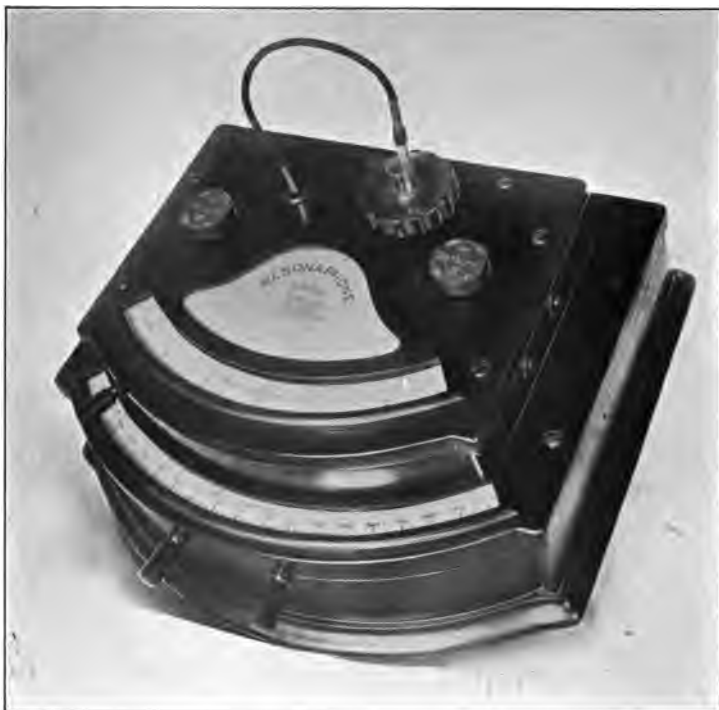
FIG. 13.—DETECTOR MOUNTED ON WAVE METER.
